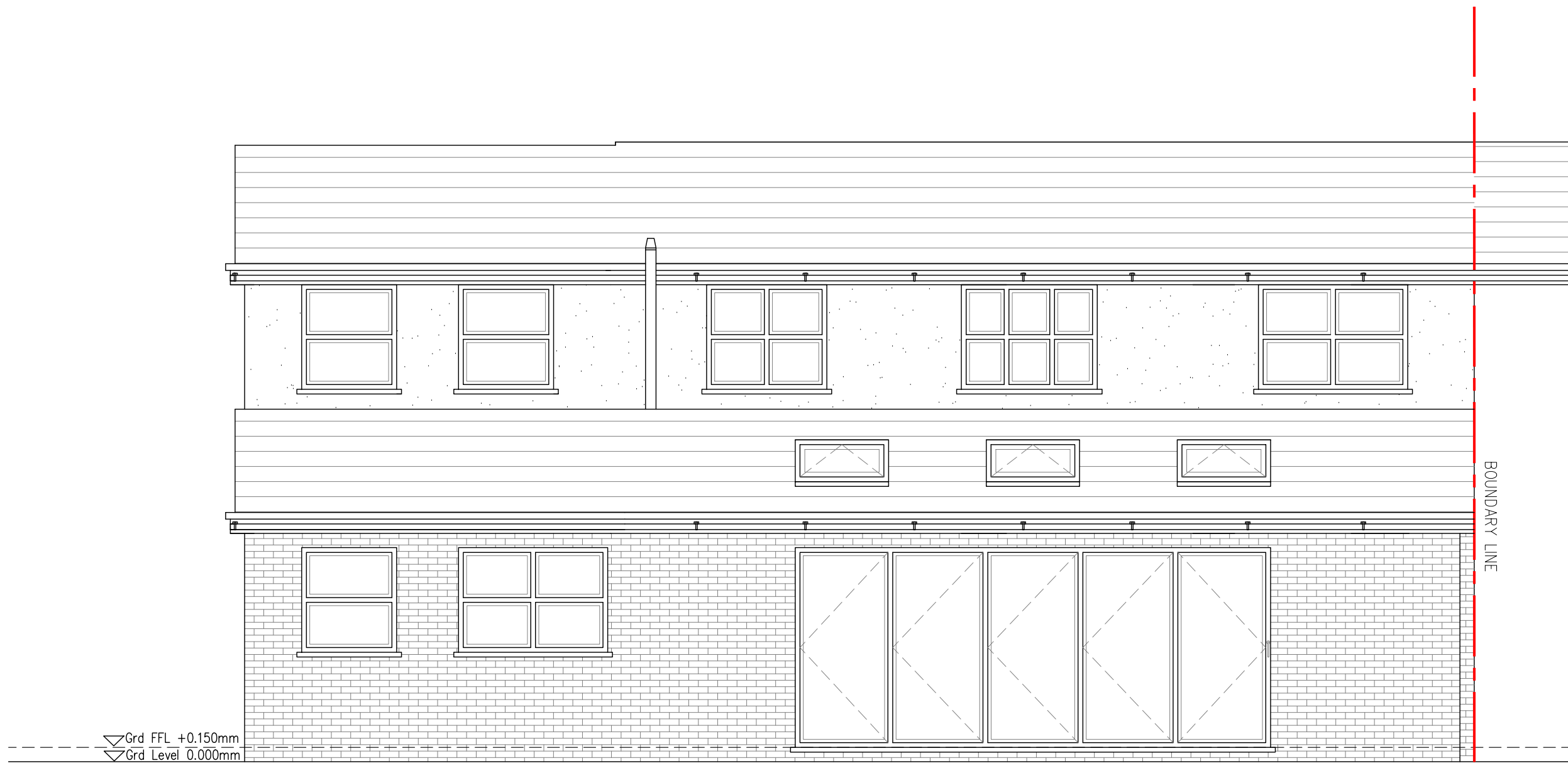
PROPOSED REAR ELEVATION | SCALE 1:50
