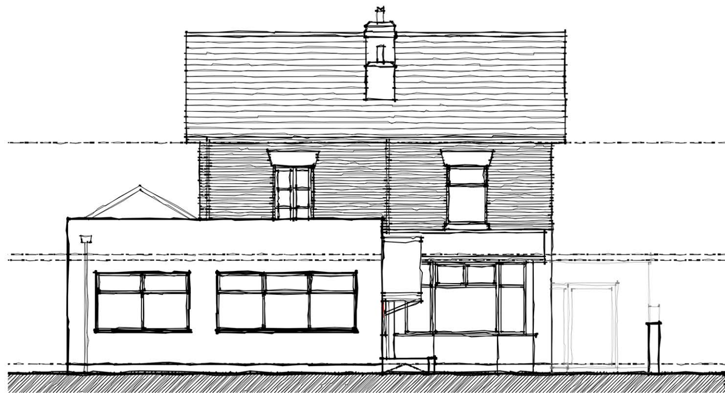
Existing Cronlon Road Elevation Scale 1:100
