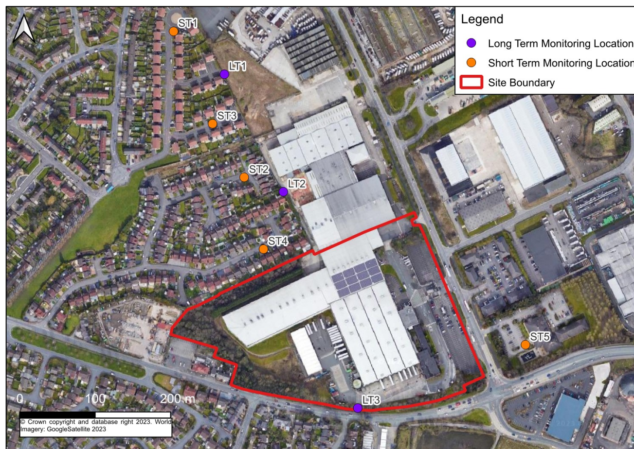
Figure 4.1: Noise Monitoring Locations
