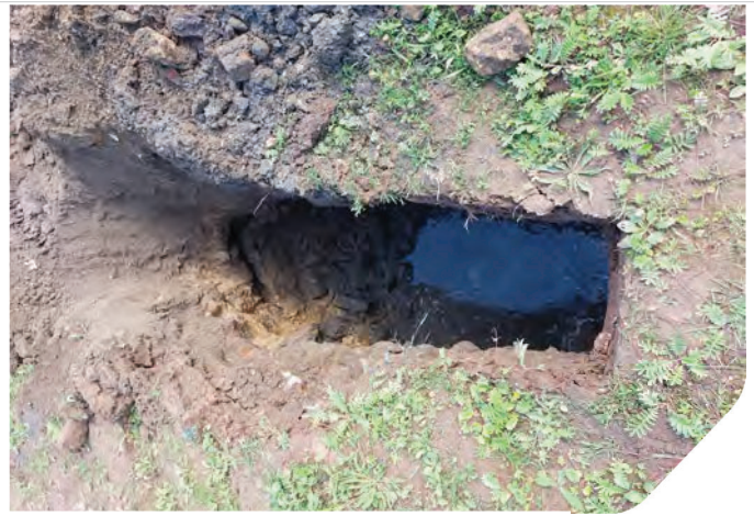
Photo 08: View of water strike within excavated TP07
