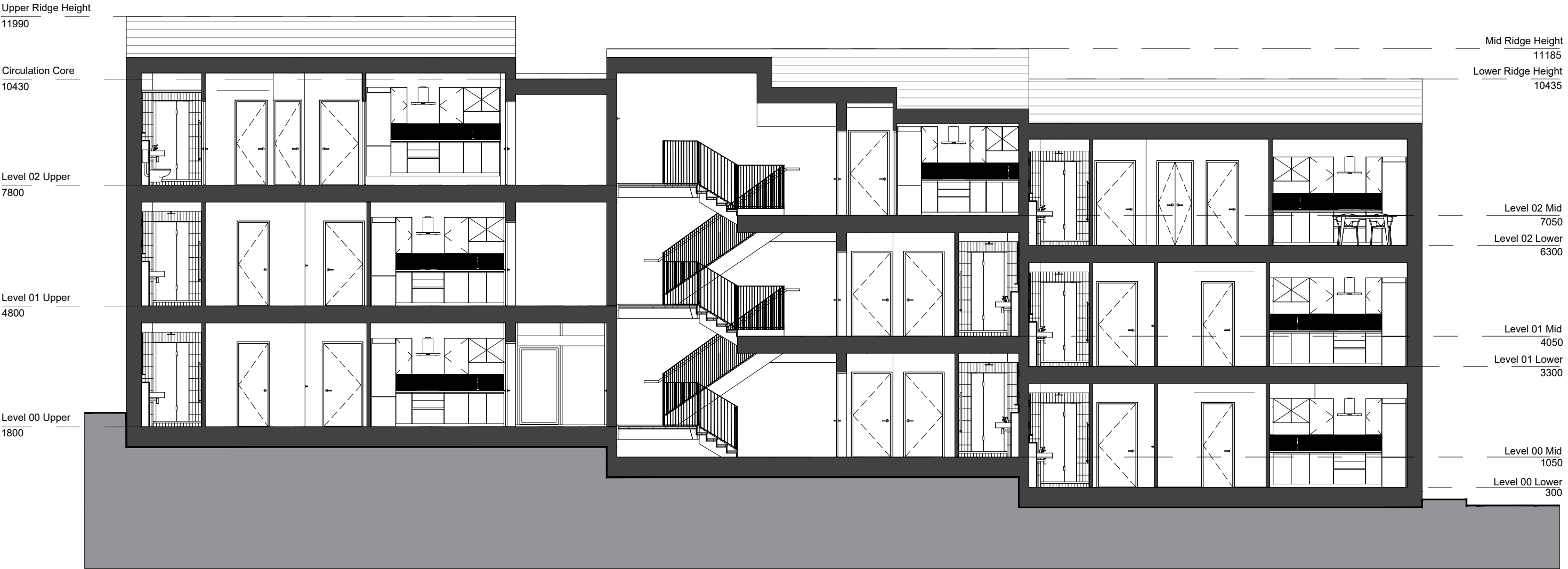
Section D-D Apartment/ Stair core/ Apartment
