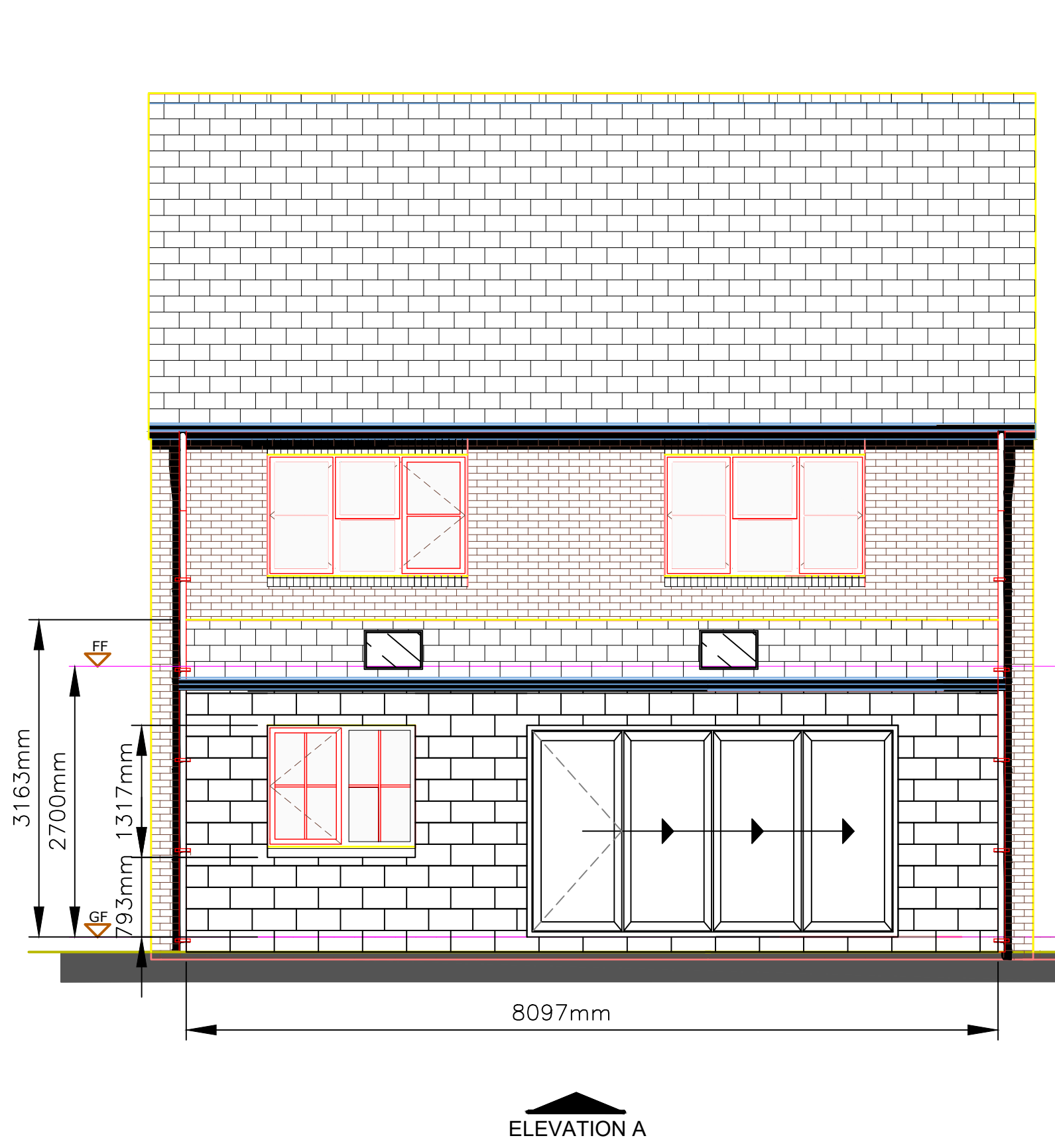
A PROPOSED BUILDING LAYOUT - ELEVATION A Scale: 1:50
