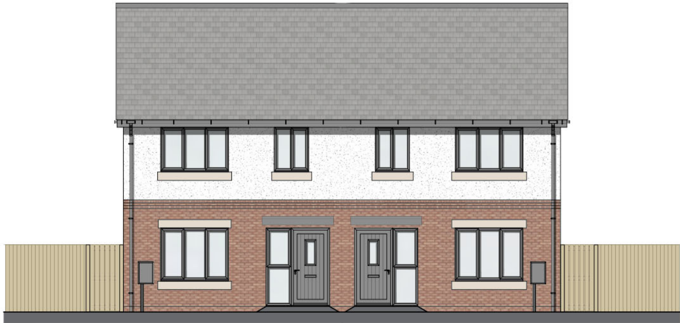
TYPE E M4(3) Adaptable 2B3P 101 (AS) FRONT ELEVATION
