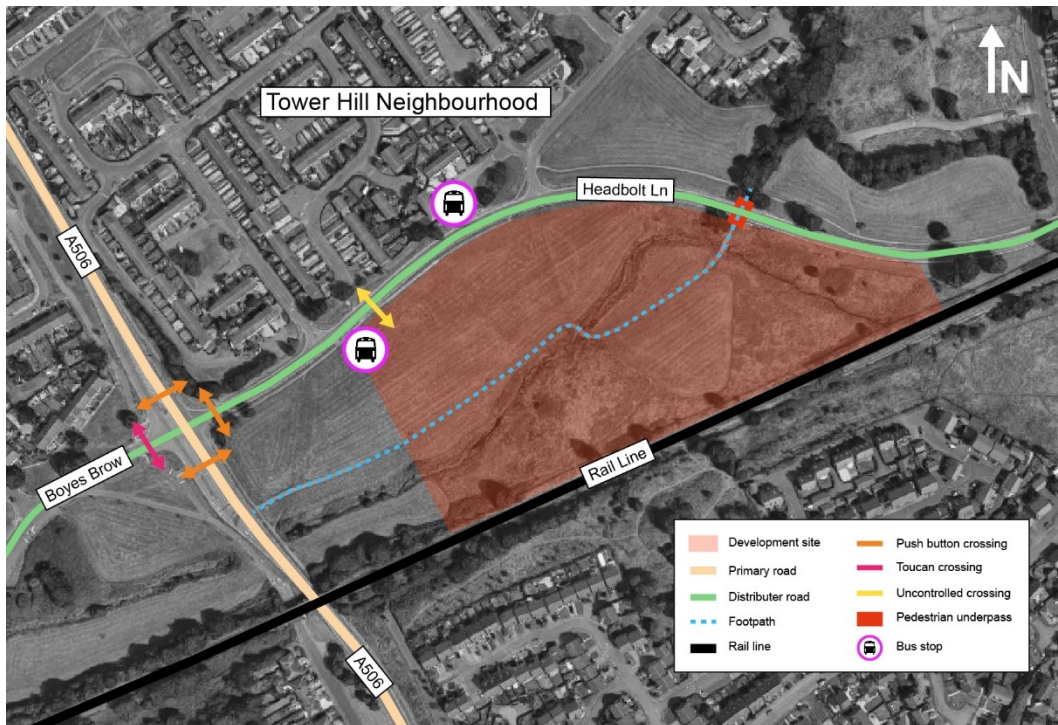
Figure 4: Key transport infrastructure
