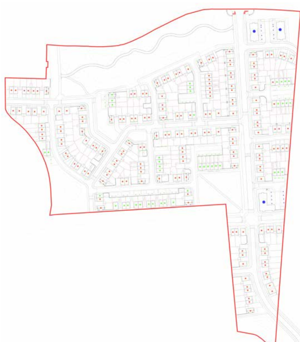
FIGURE 41: ELECTRIC VEHICLE CHARGING
