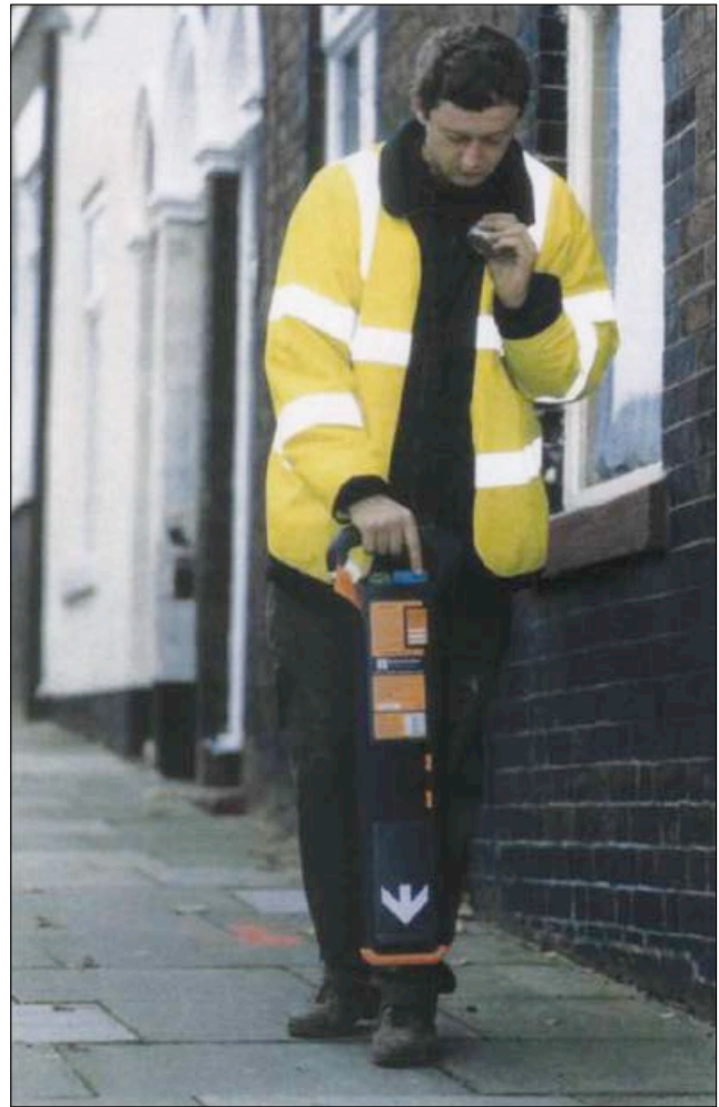
Figure 5 Using a cable locator
