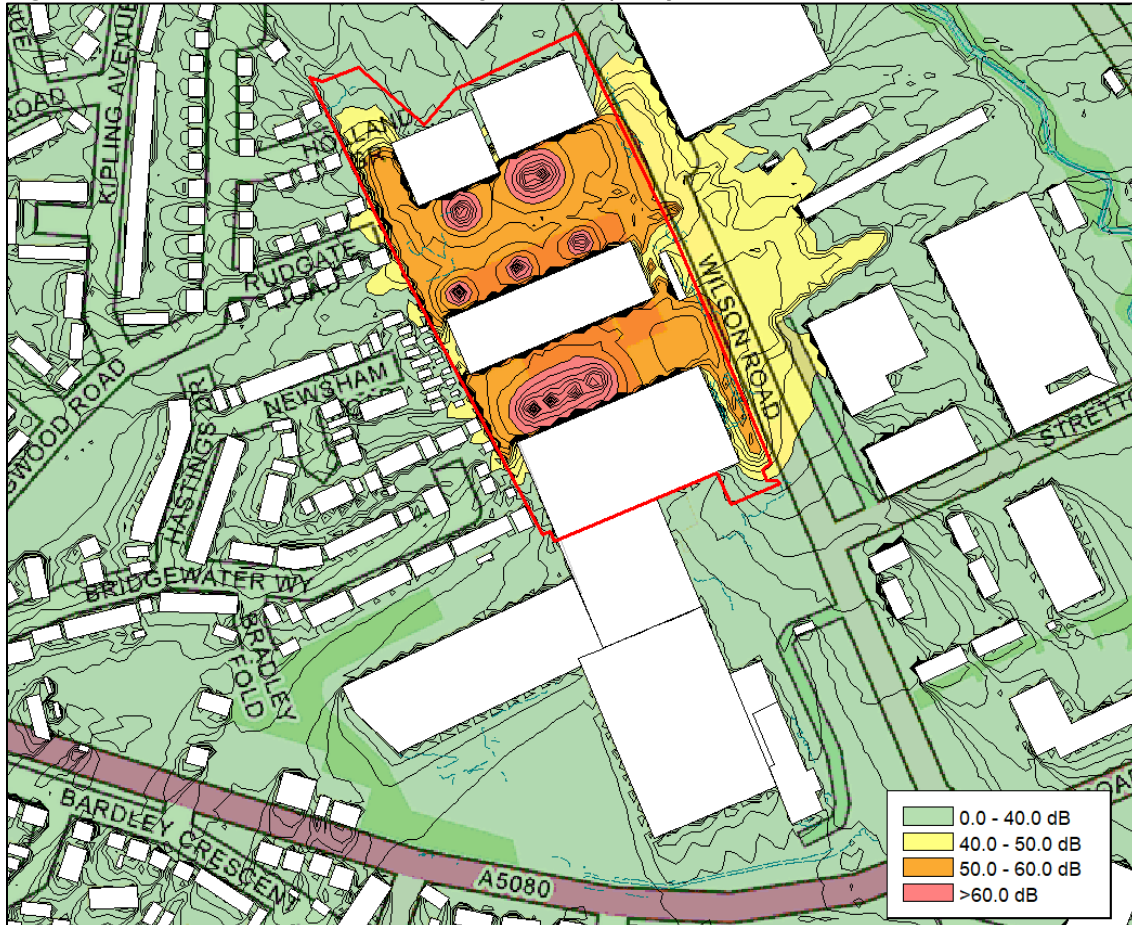
Figure 5.2 Noise Contour Plot Daytime ( L_{Aeq,1hour} )
