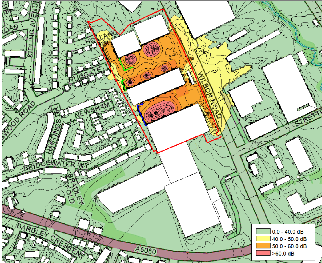
Figure 6.2 Noise Contour Plot Daytime ( L_{Aeq,1hour} ) – Including Mitigation
