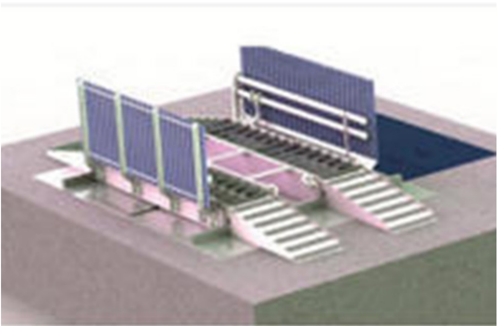
Figure 19. Example of type of MAIN wheel wash enclosure to be used
