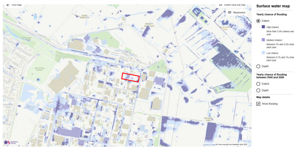
Figure 4.7a Environment Agency – Existing Pluvial Flood Map
