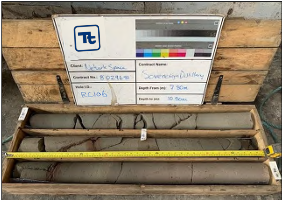
Photo Plate No. 15: RC106 4.80-10.80m
