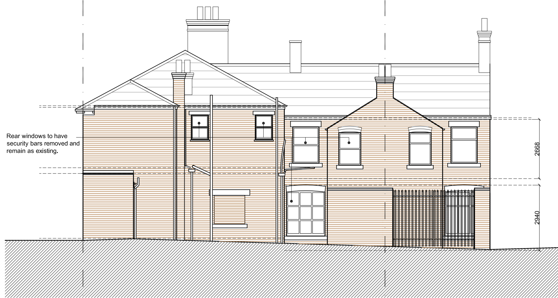
Proposed Rear Elevation Scale 1:100
