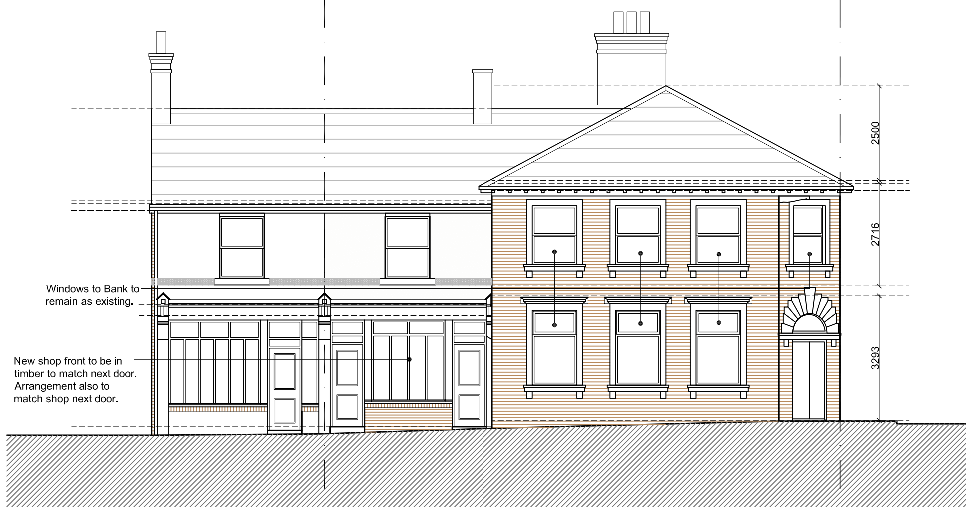
Proposed High Street Elevation Scale 1:100
