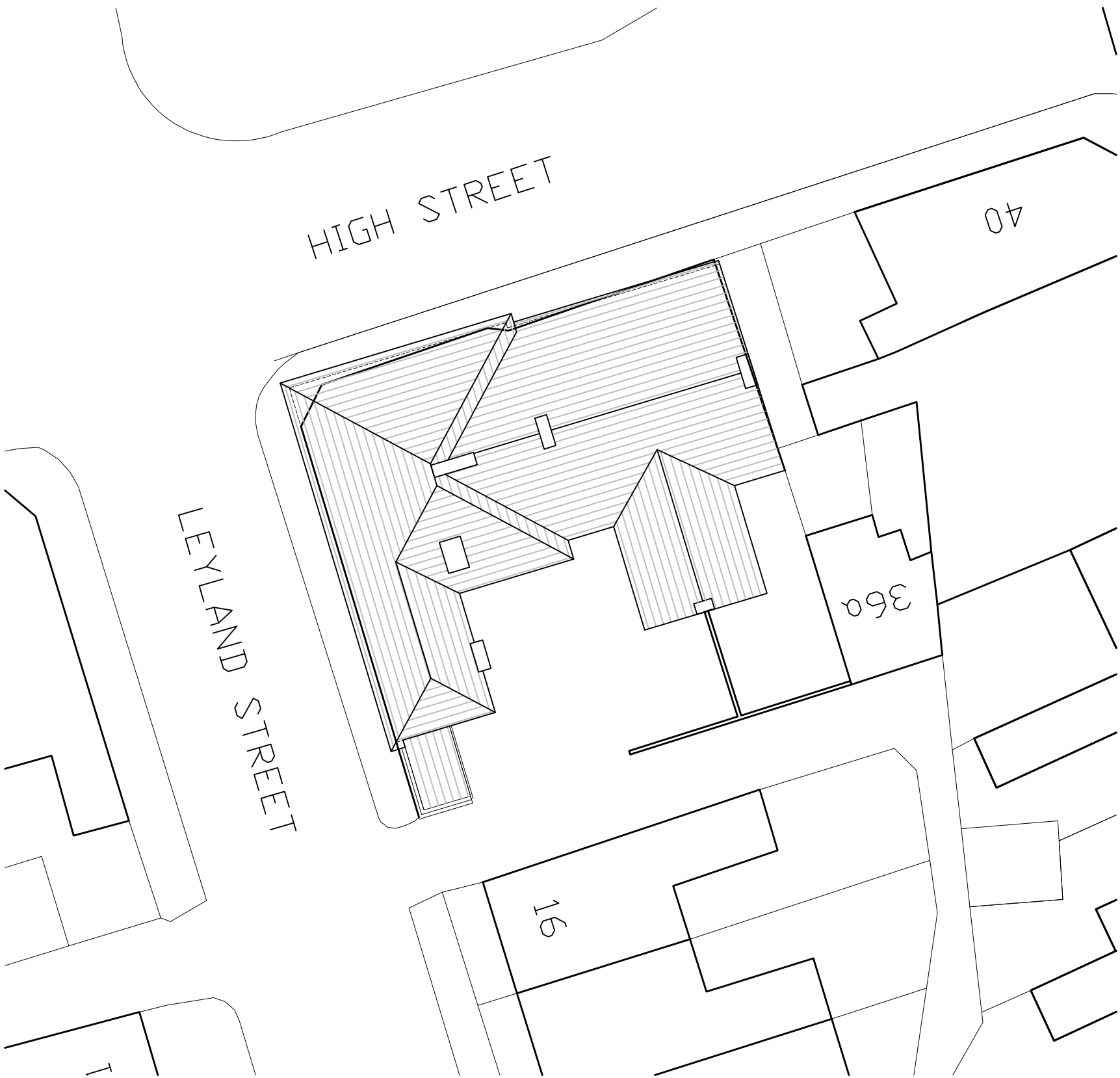
Proposed Site Plan (Roof Layout) Scale 1:200
