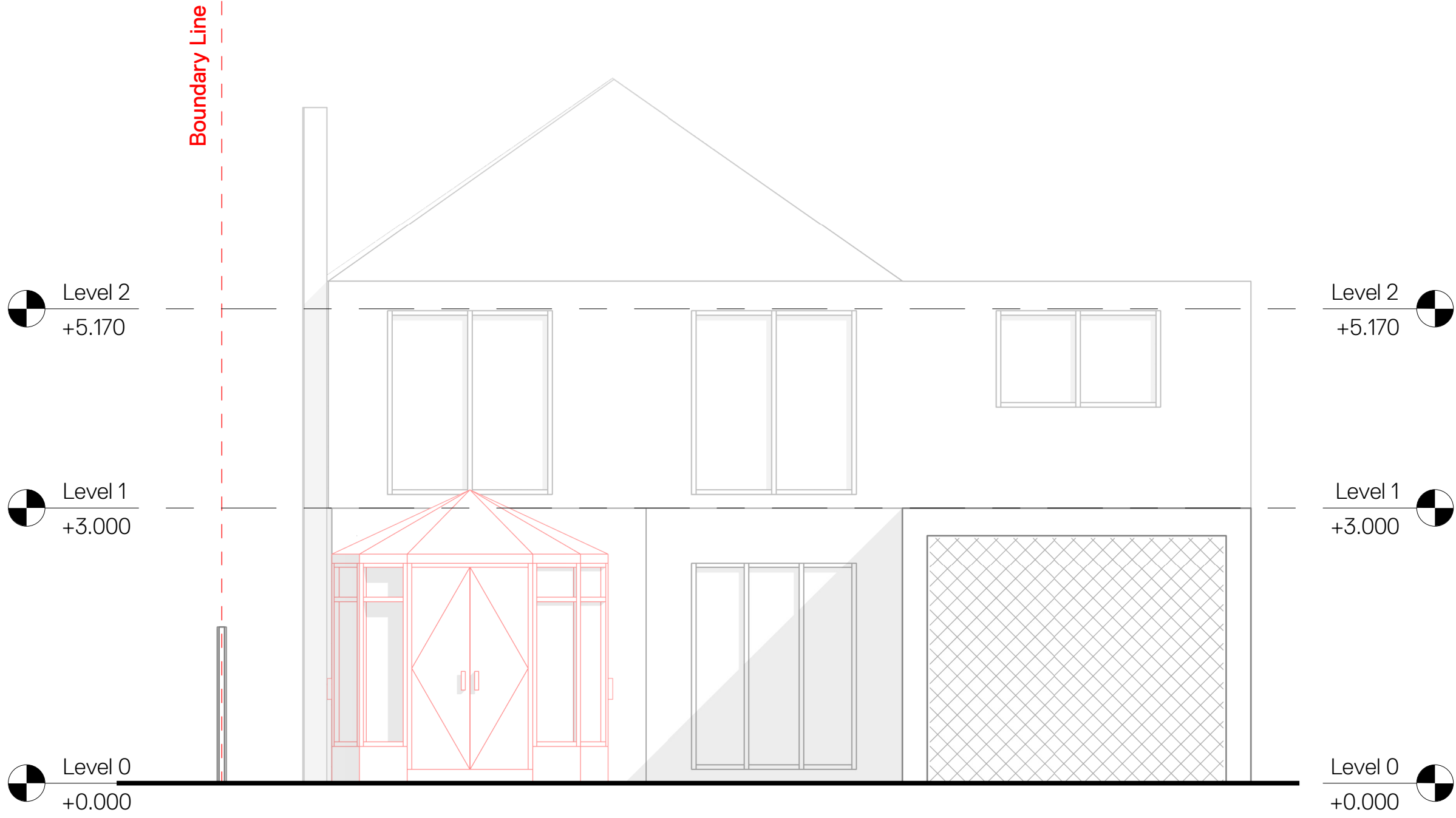
A Demolition Garden Elevation 1: 50
