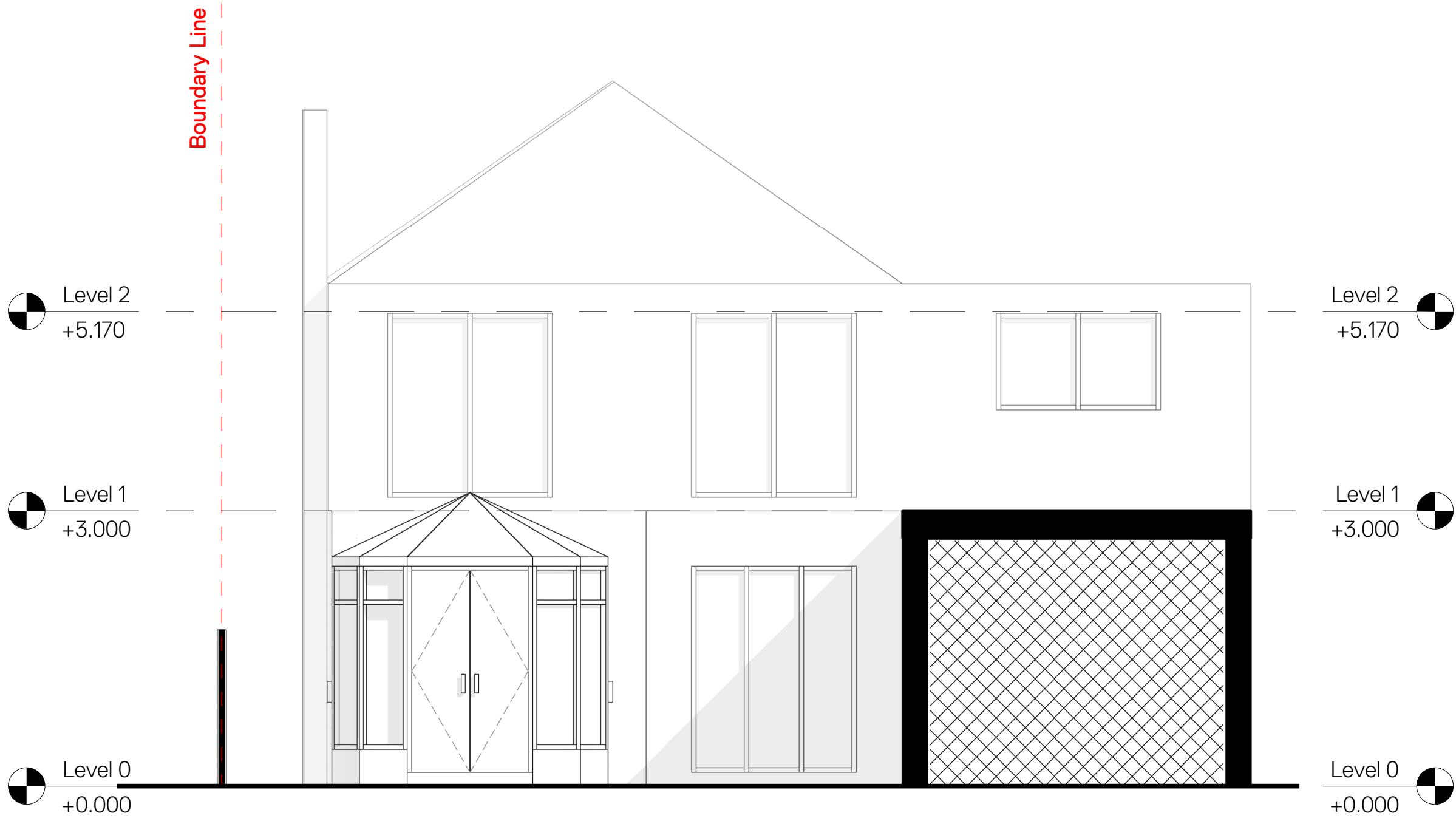
A Existing Garden Elevation 1: 50
