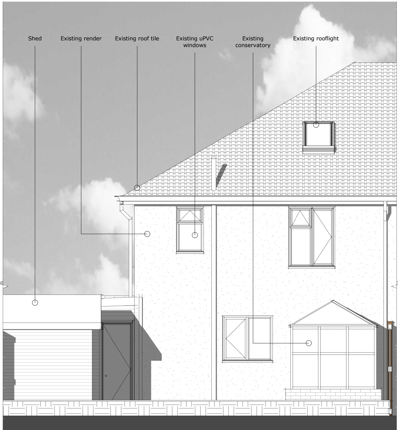
3 Existing Rear Elevation
