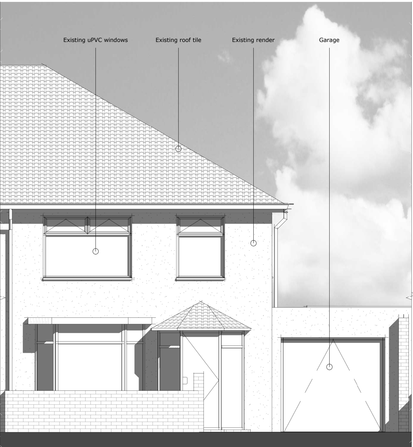
1 Existing Front Elevation
