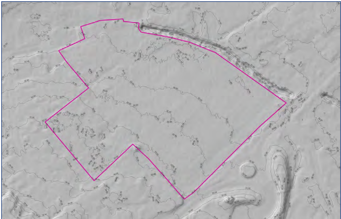
Figure 5: An extract of the LiDAR imagery of the site, showing the relatively flat nature of the site. The dip in topography to the north of the site boundary is consistent with the presence of the River Alt.
