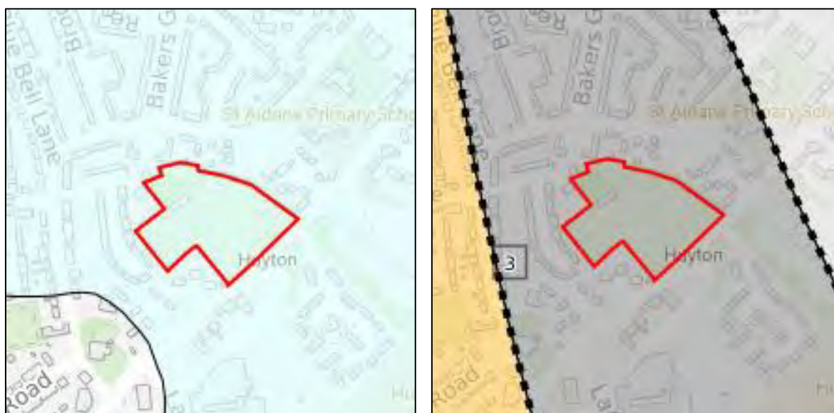
Figure 13: Extracts of the BGS 1:50,000 drift (left) and solid (right) geological maps. Light blue = Glacial Till, Dark grey and light grey = Pennine Middle Coal Measures Formation, Light grey = Chester Formation.
