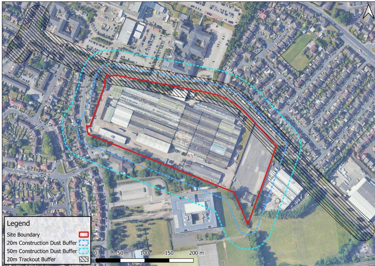
Figure 4: Construction Dust Buffers
