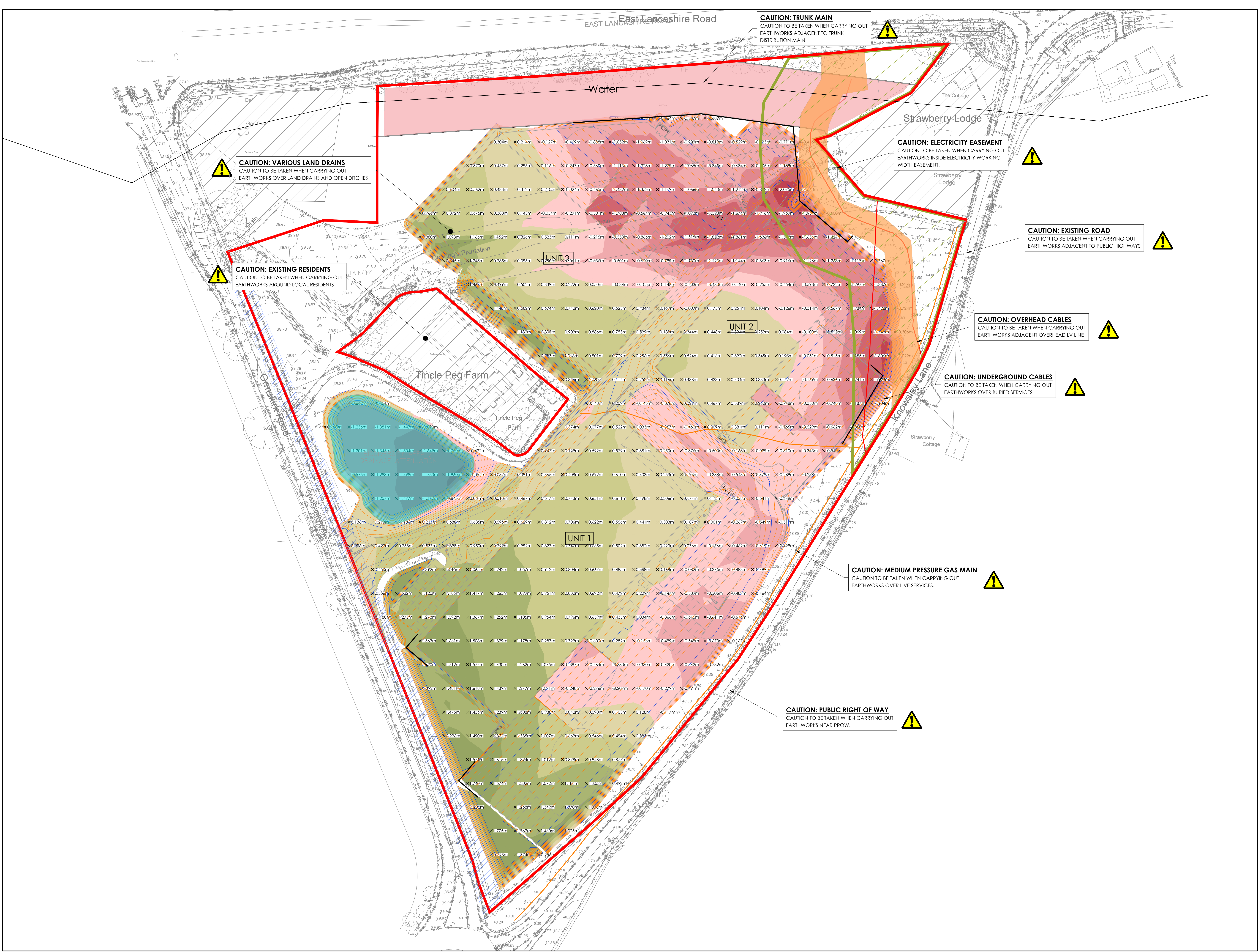
JPG-PROPOSED EARTHWORKS - CUT & FILL ANALYSIS
