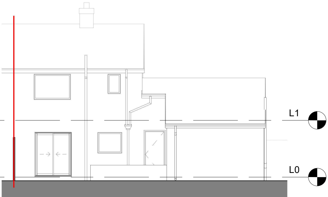
3 Rear Elevation as Existing 1 : 100
