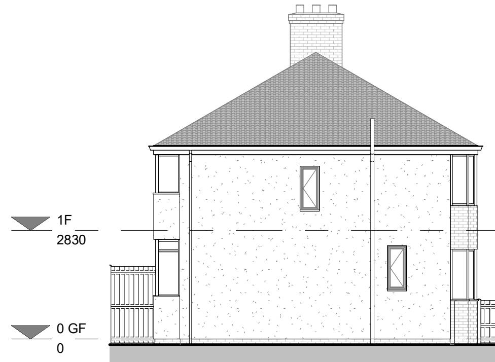
EXISTING SIDE ELEVATION II SCALE 1:100@A3
