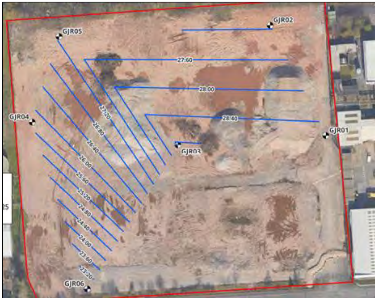
Figure 4.2 Chester Formation Groundwater Contours
