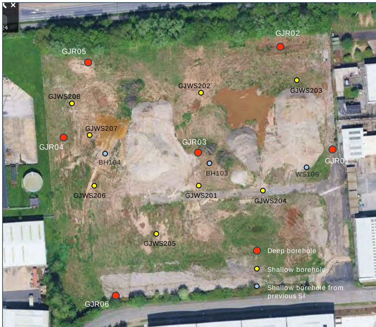
Figure 4.1. Supplementary Works – Standpipe Locations
