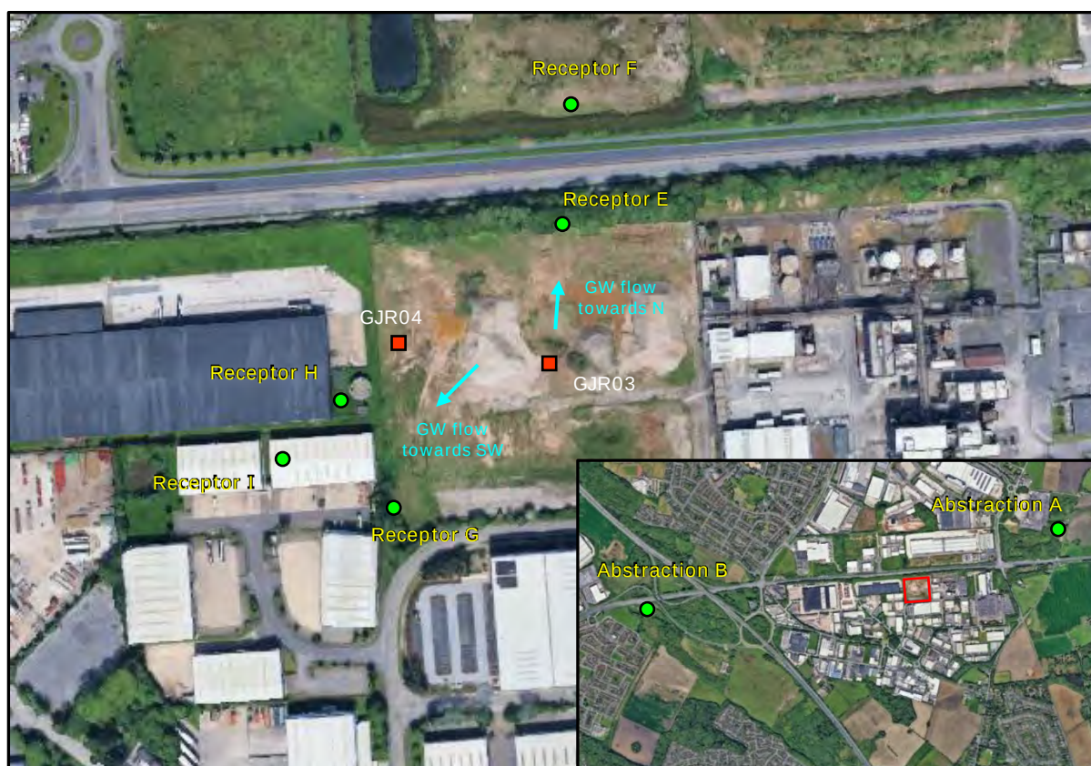
Figure 6.2 Modelled Groundwater Source Areas and Receptors
