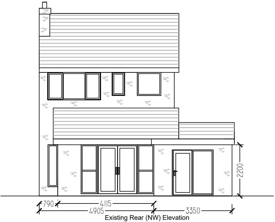
Existing Rear (NW) Elevation
