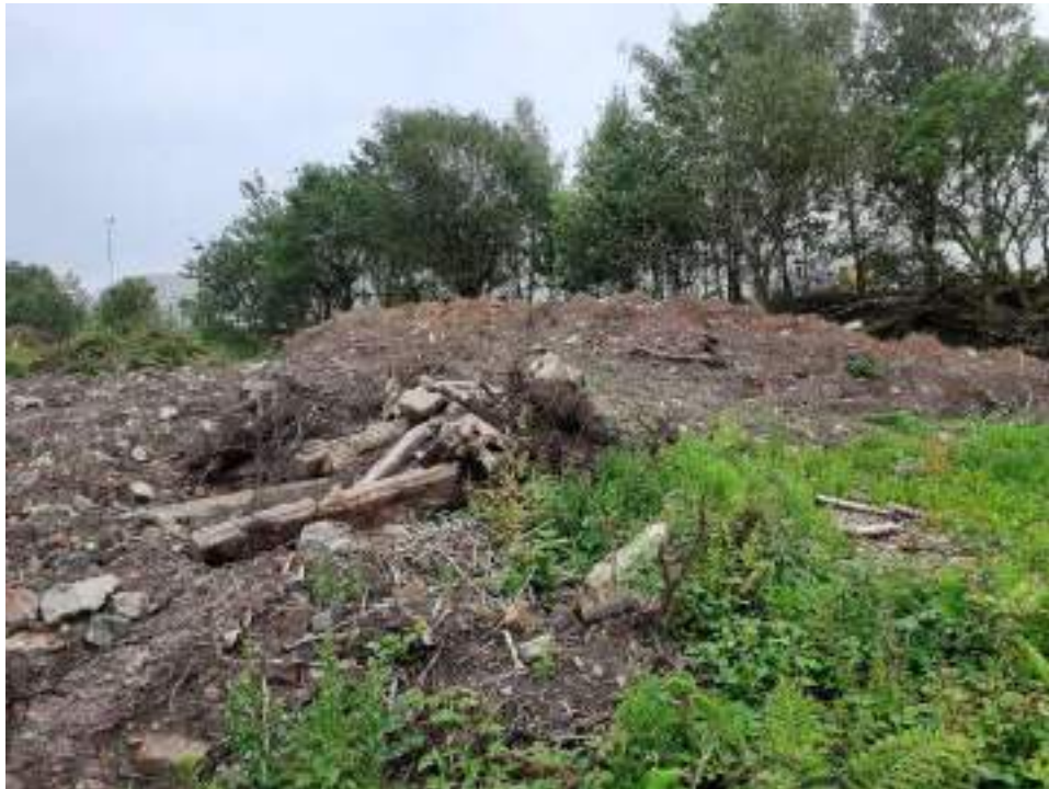
Photo 3: Stockpile of predominantly granular material with inclusions of brick and concrete cobbles / boulder located in the south.
