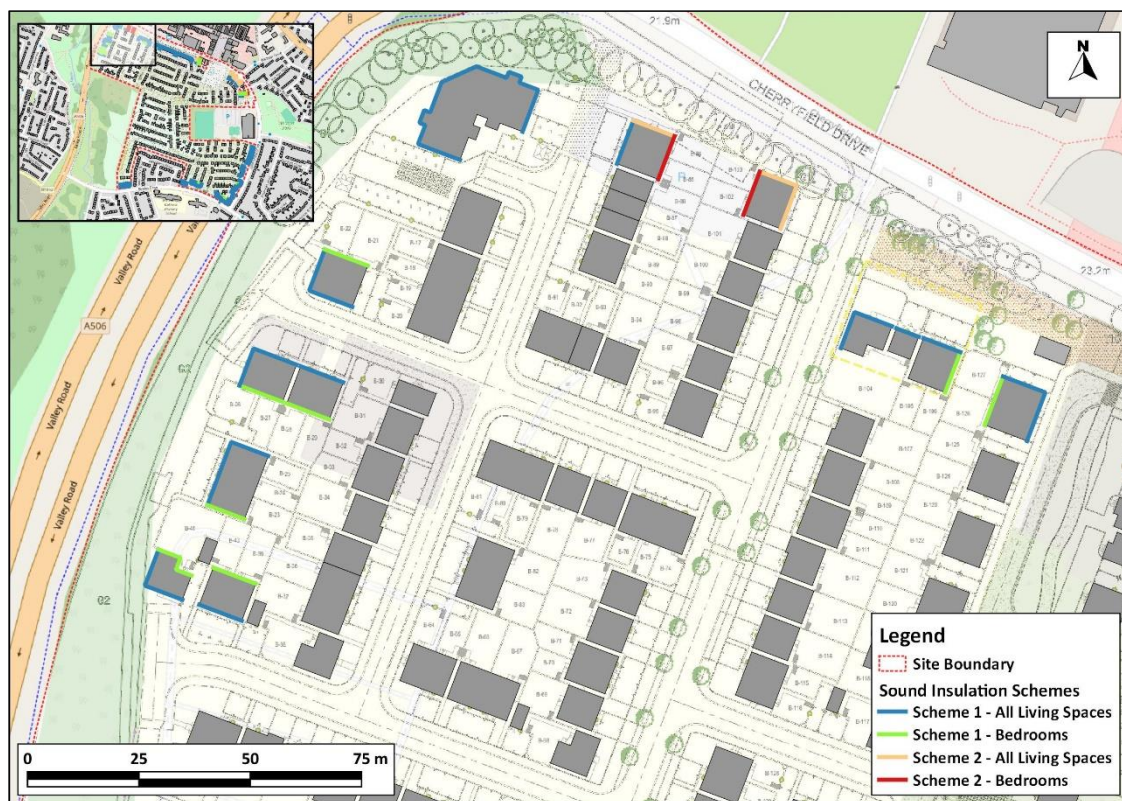
Figure 8.3.11: Recommended Road Traffic Sound Insulation Scheme [1]
