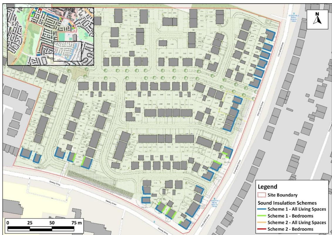
Figure 8.3.14: Recommended Road Traffic Sound Insulation Scheme [4]
