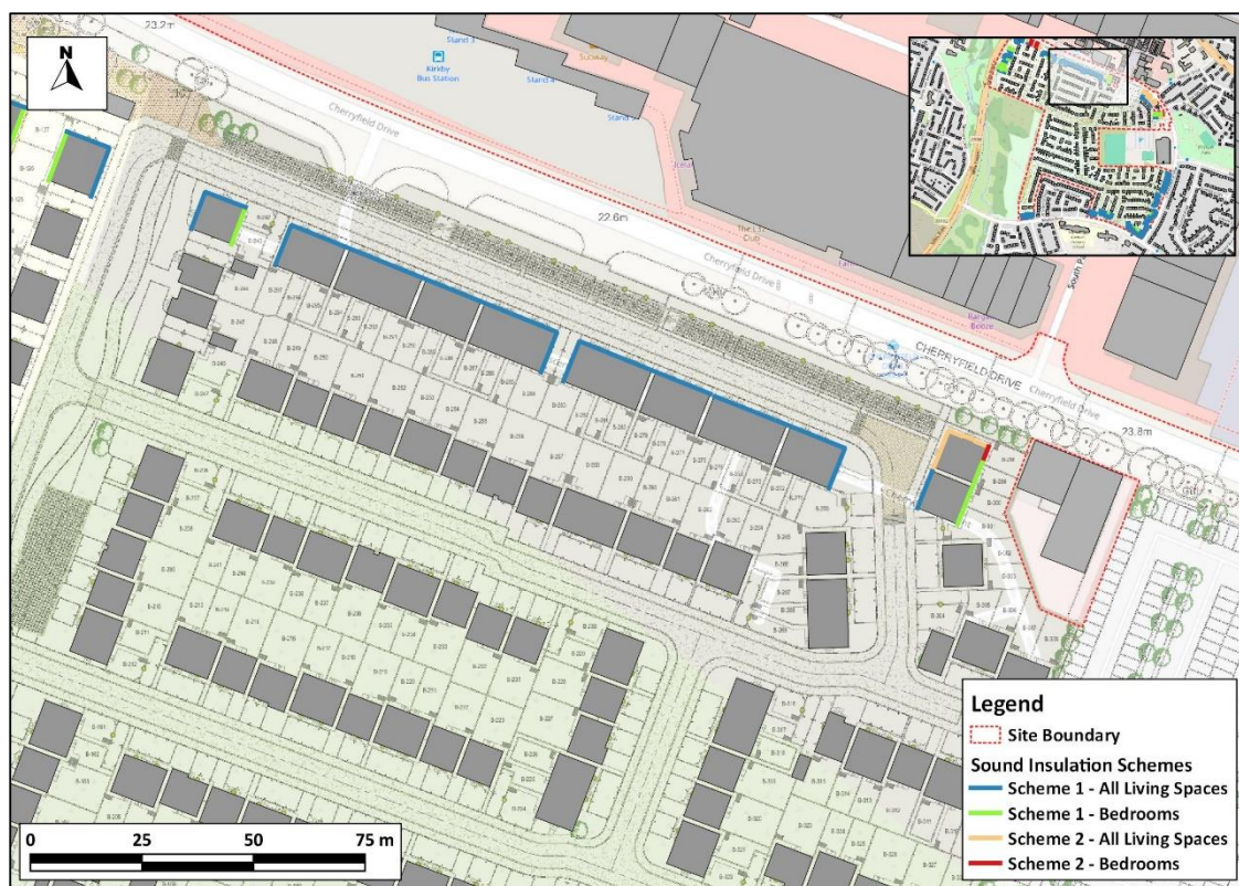
Figure 8.3.12: Recommended Road Traffic Sound Insulation Scheme [2]
