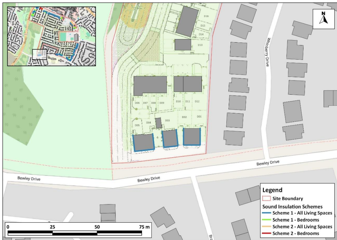
Figure 8.3.15: Recommended Road Traffic Sound Insulation Schemes [5]
