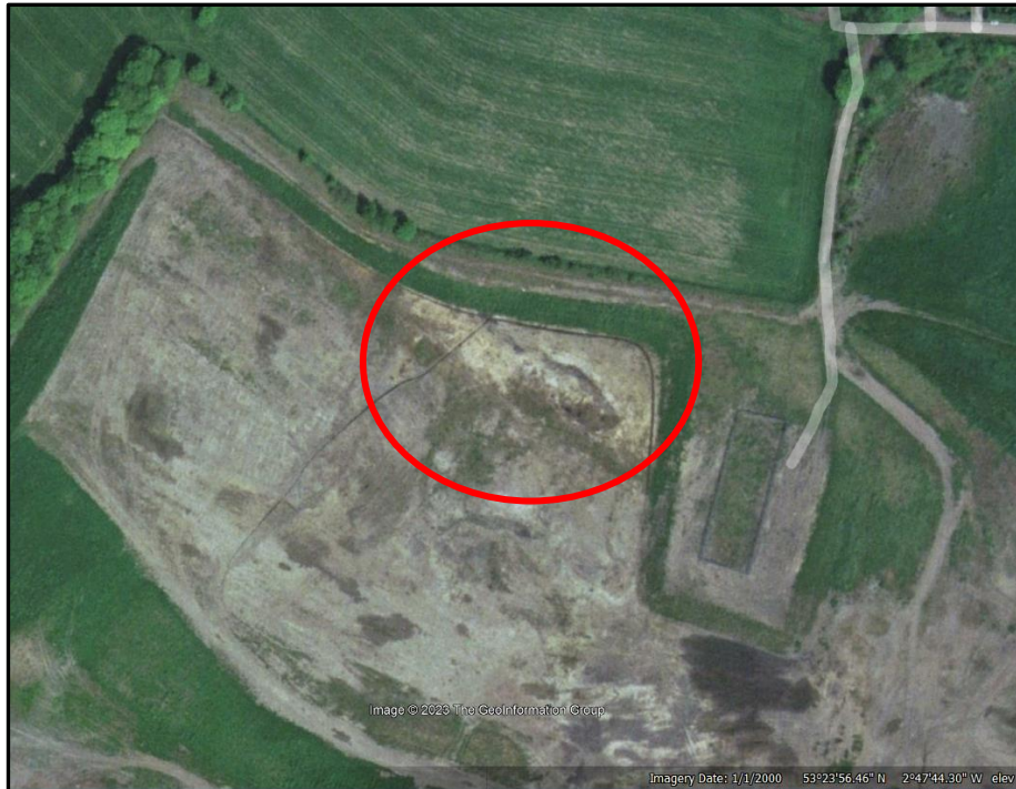
Figure 6-2 Historic Aerial Image Showing Potential Hummocky Ground
