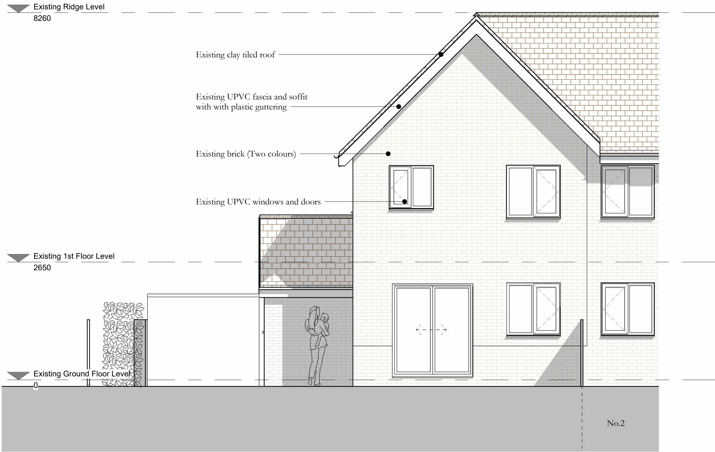
Existing Rear (North West) Elevation
