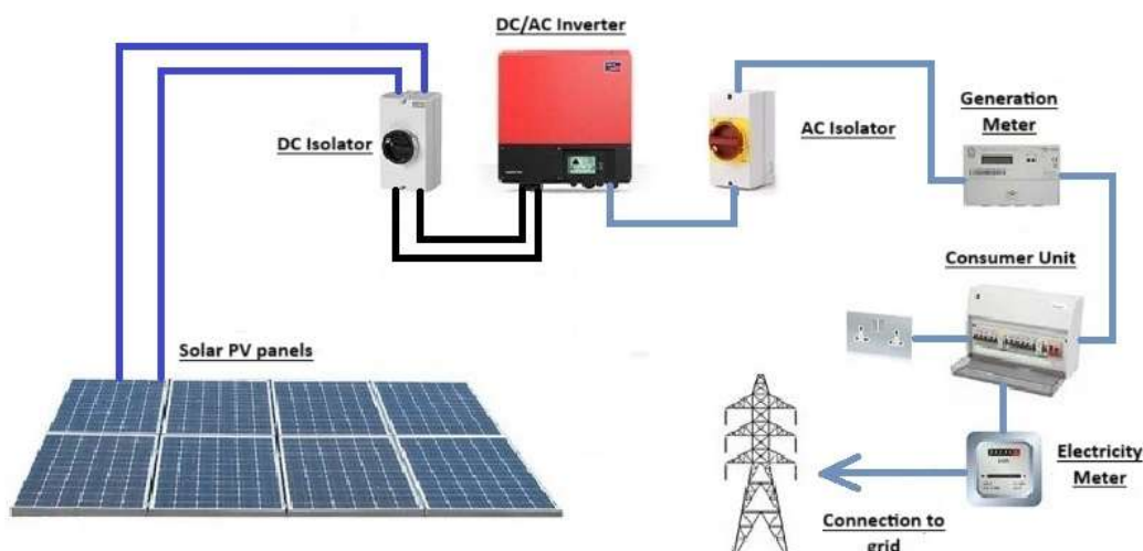
Figure 6 – Photovoltaic Panels – Typical Diagram
