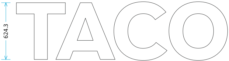
3mm opal 050 faces made 5mm smaller a/r
