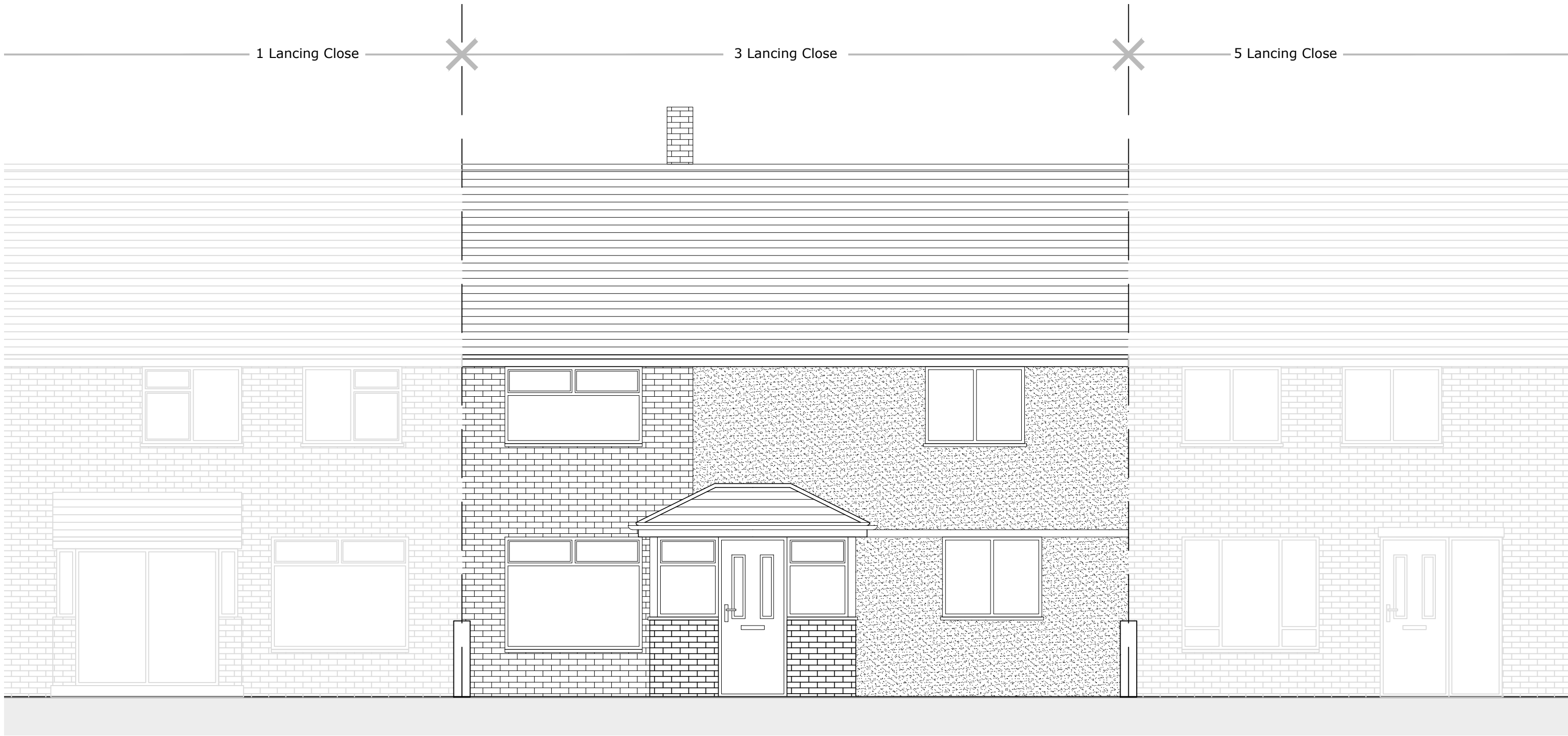
front elevation (east facing) as existing 1:50
