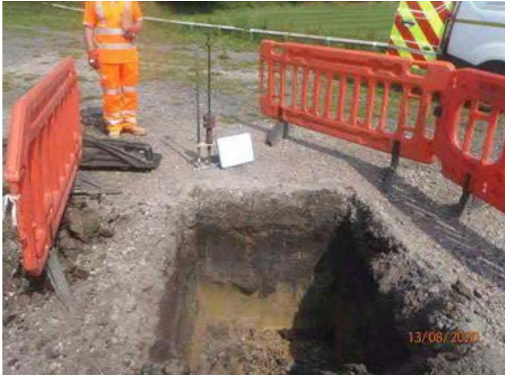
PHOTO 6 SHOWING SOAKAWAY LEVEL ON 2nd DAY
