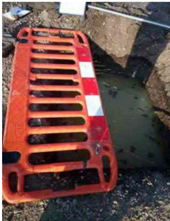
PHOTO 6 SHOWING SOAKAWAY LEVEL ON 2nd DAY
