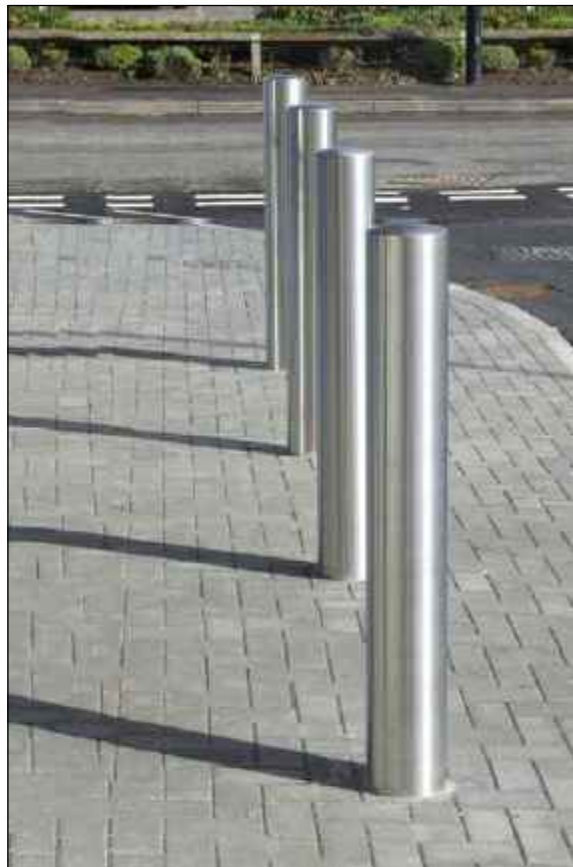
Bollard Type 1 - Impact protection Steel posts, 1100mm high. Concrete filled, stainless steel. Bolted to concrete hardstand.
