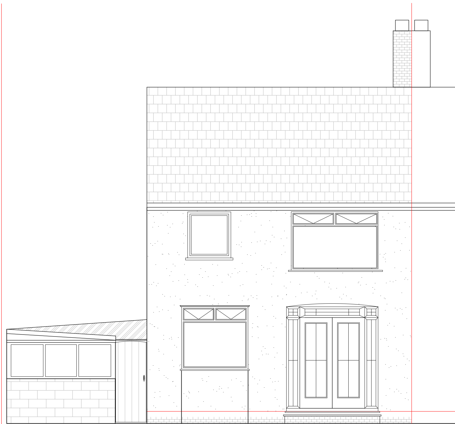
Existing Rear Elevation. (C - C) Scale 1:50 @A1
