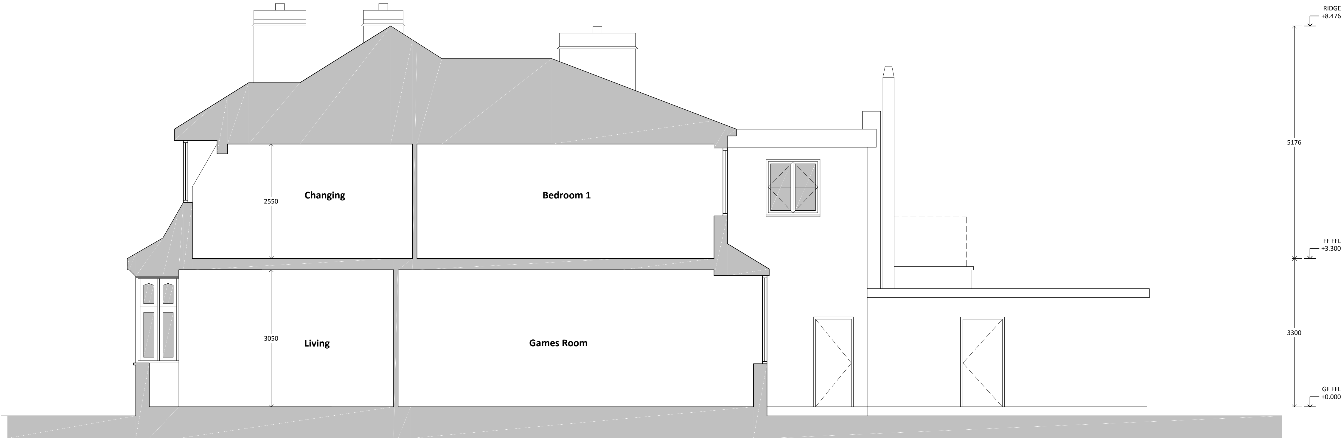
EXISTING SECTION A-A SCALE 1:50
