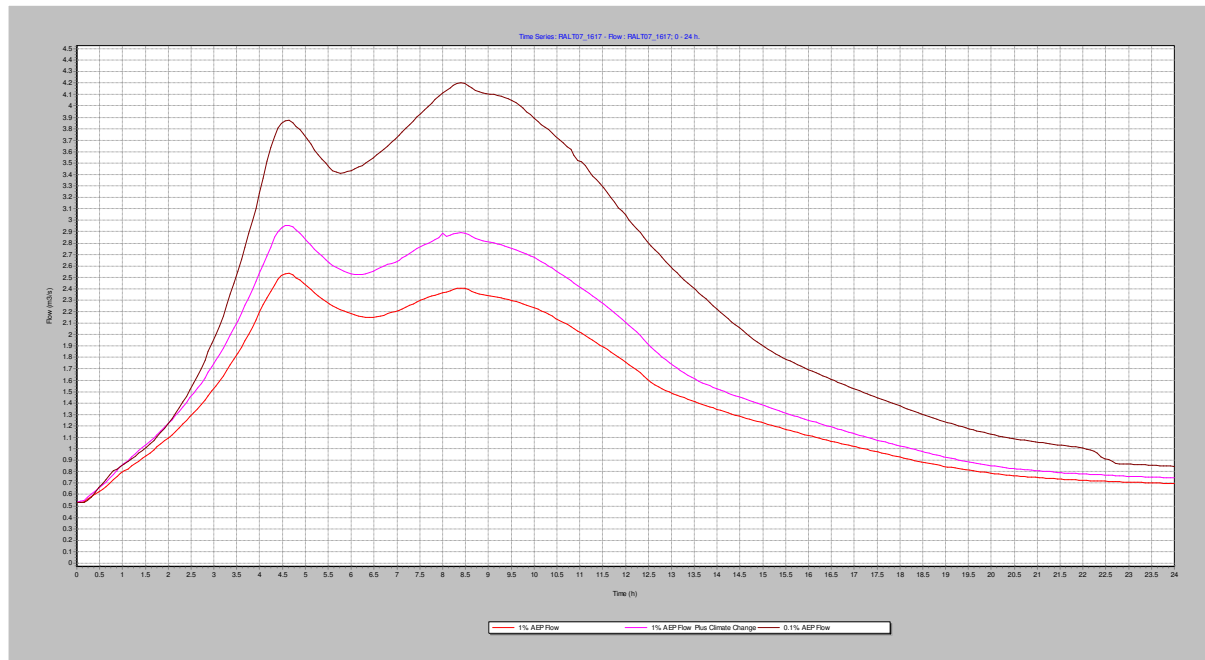
Figure D.1 Upstream flows for the 1%, 1% climate change and 0.1% AEP events
