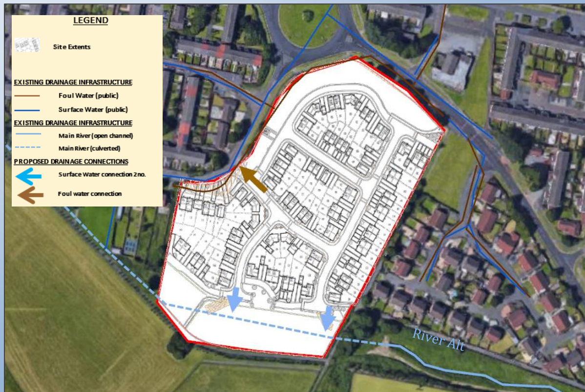
Figure 8: Preliminary Drainage Strategy (Betts Hydro 2018)
