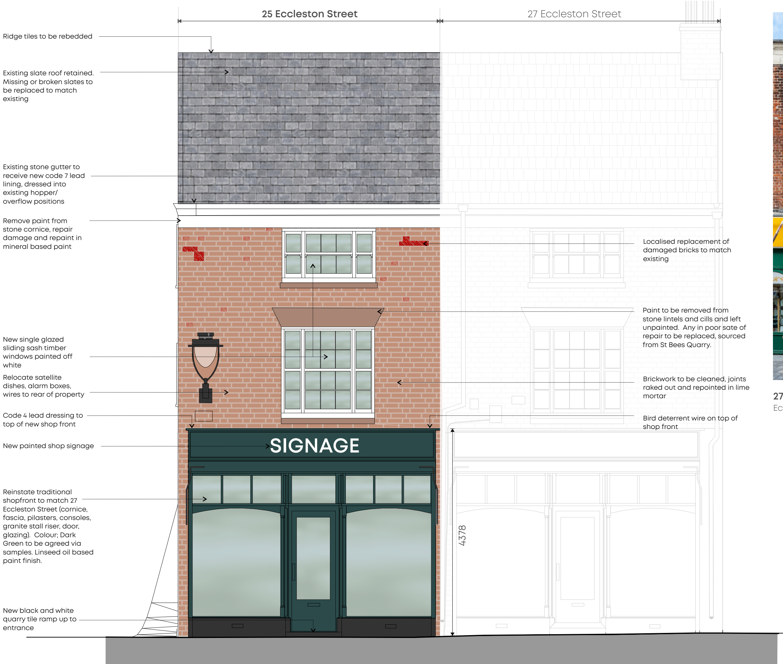
Front Elevation scale 1:50
