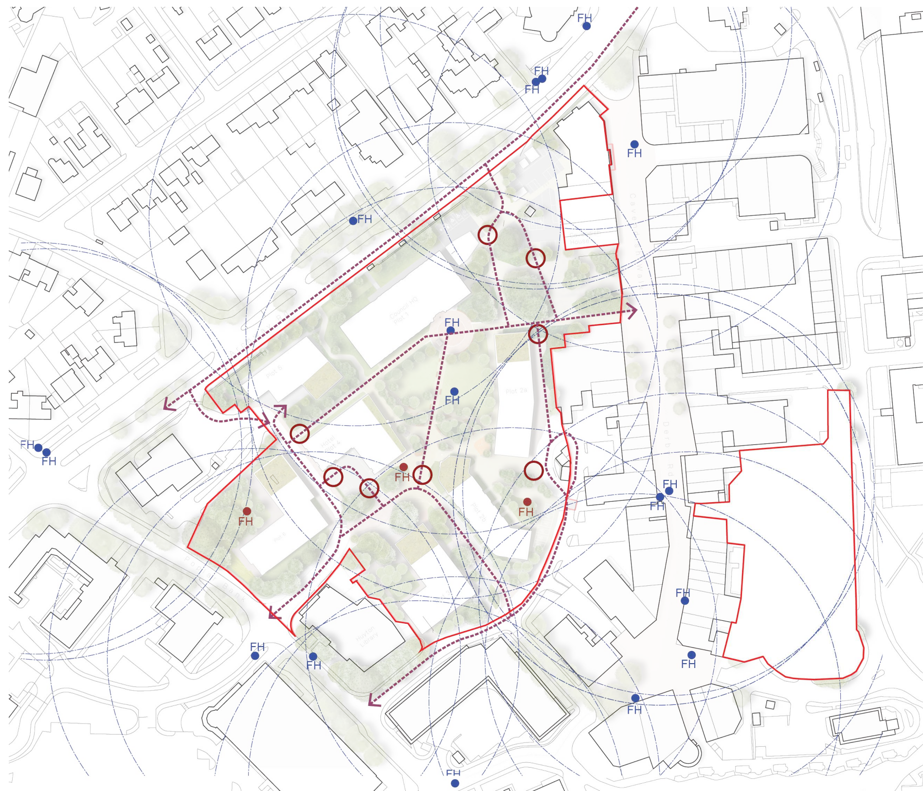
Figure 113: Fire hydrant location and access requirements plan
