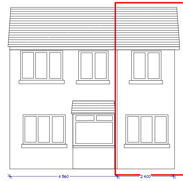
Proposed Front (SE) Elevation 1:100
