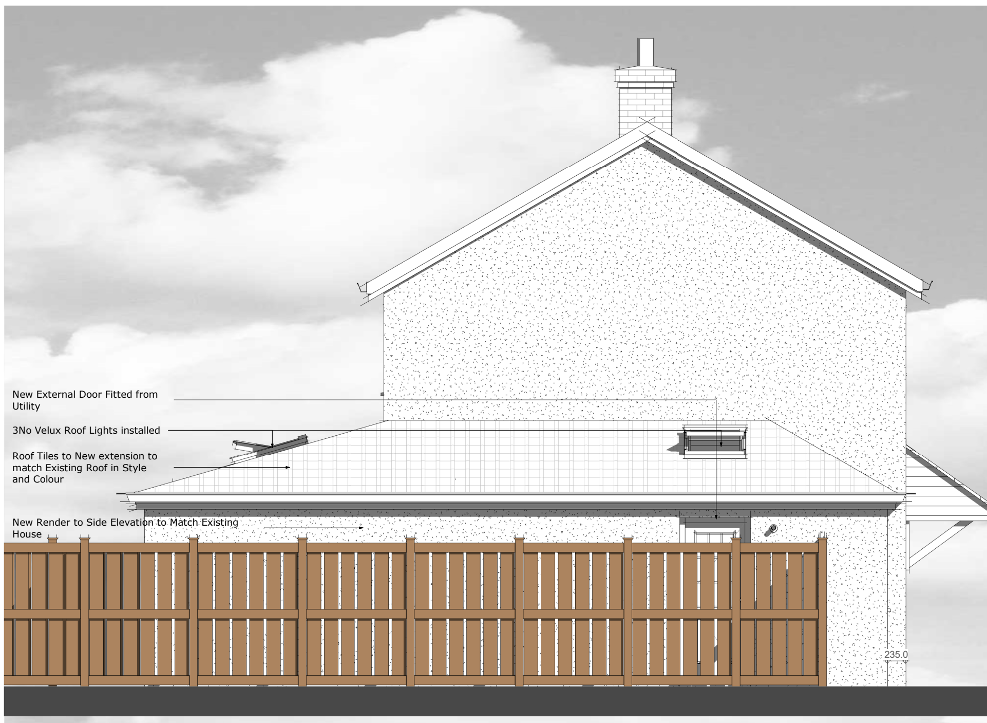
01 Proposed Side Elevation
