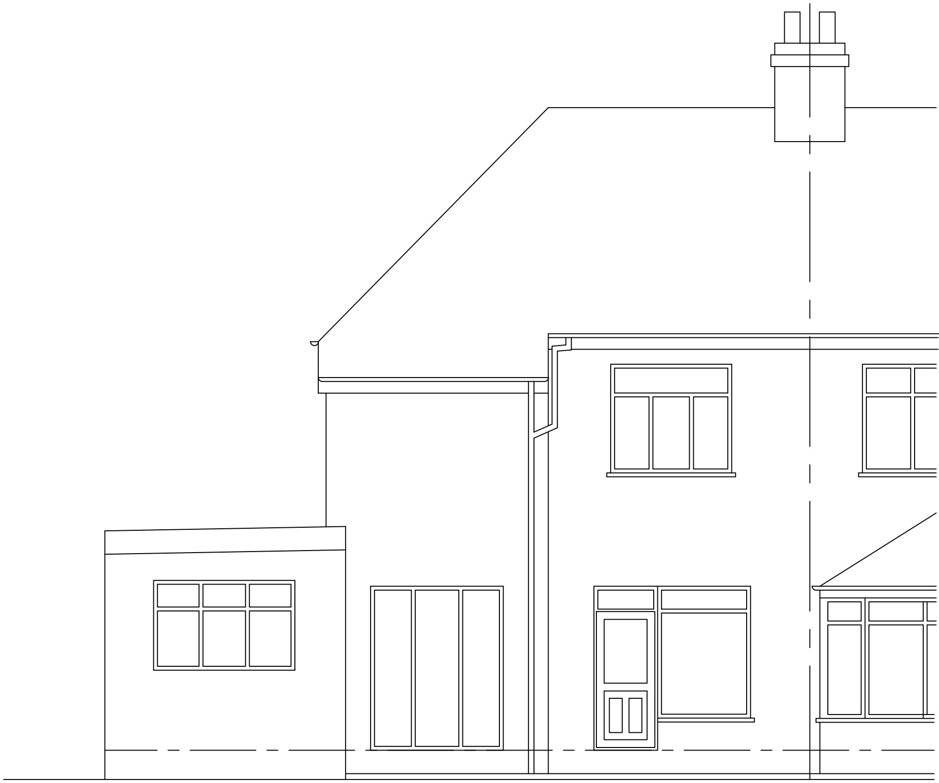
Existing Rear Elevation. (1:50)
