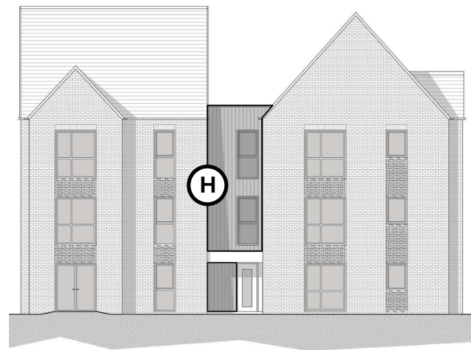
Apartment Block B - Cladded connecting element
