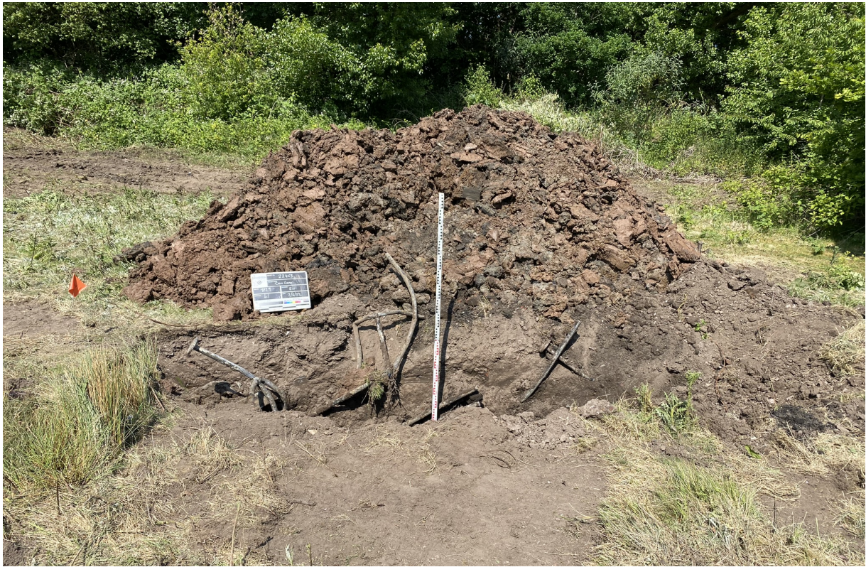
Photograph 15 – TP29 excavated to 4.1m bgl. Evidence of historic foundations.
