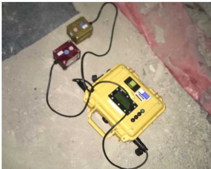
Figure 10 Vibrock Vibration Monitoring System
