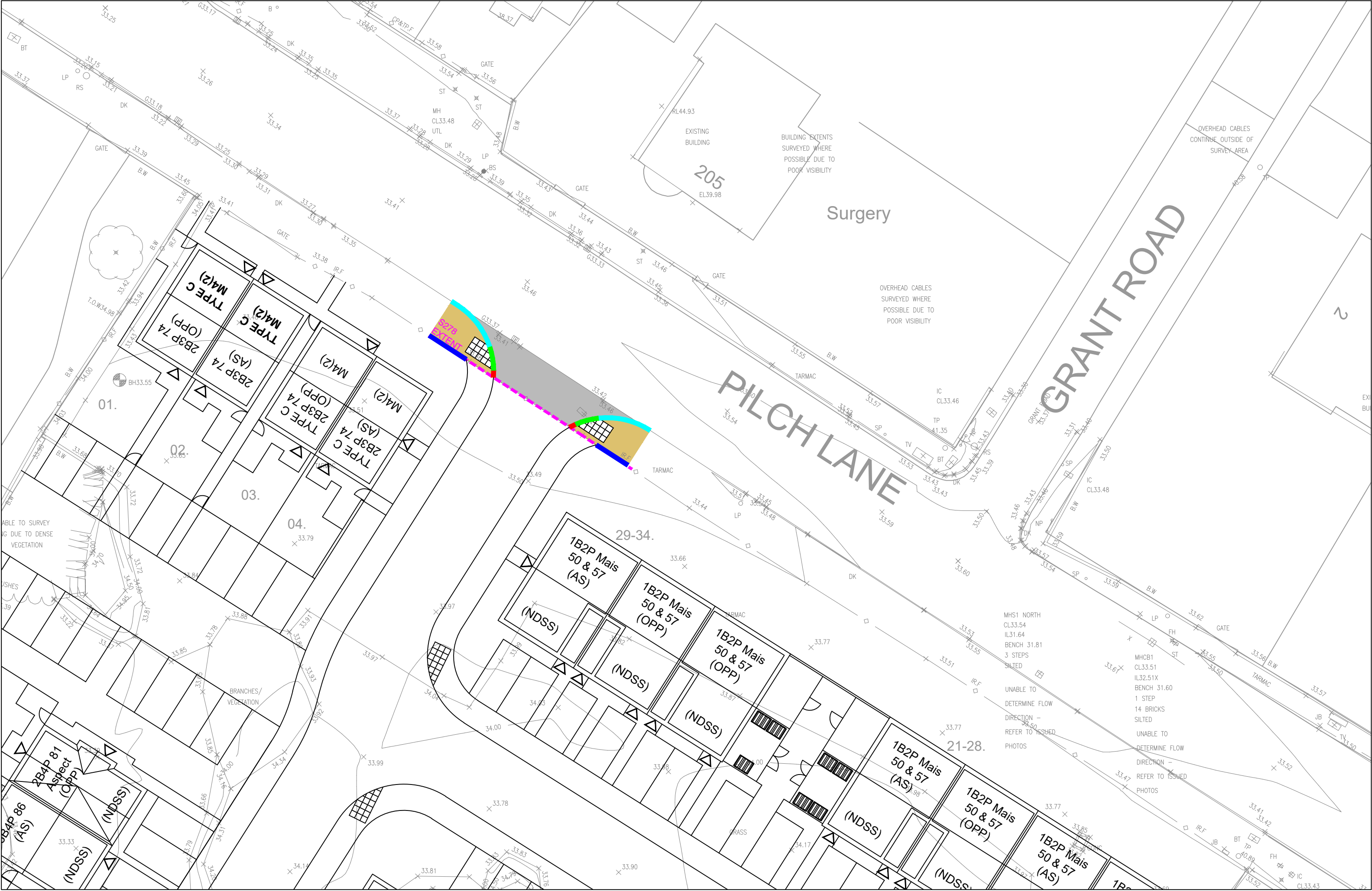
S278 Kerbing & Surfacing Layout Scale 1:250
