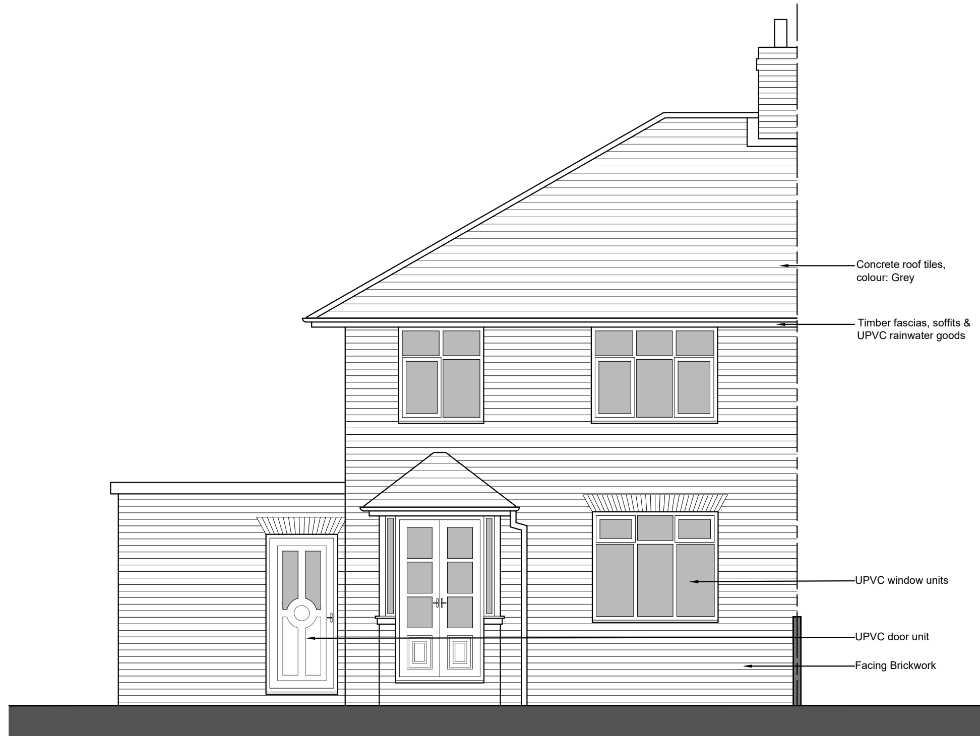
EXISTING FRONT (SOUTH-WEST) ELEVATION 1:50
