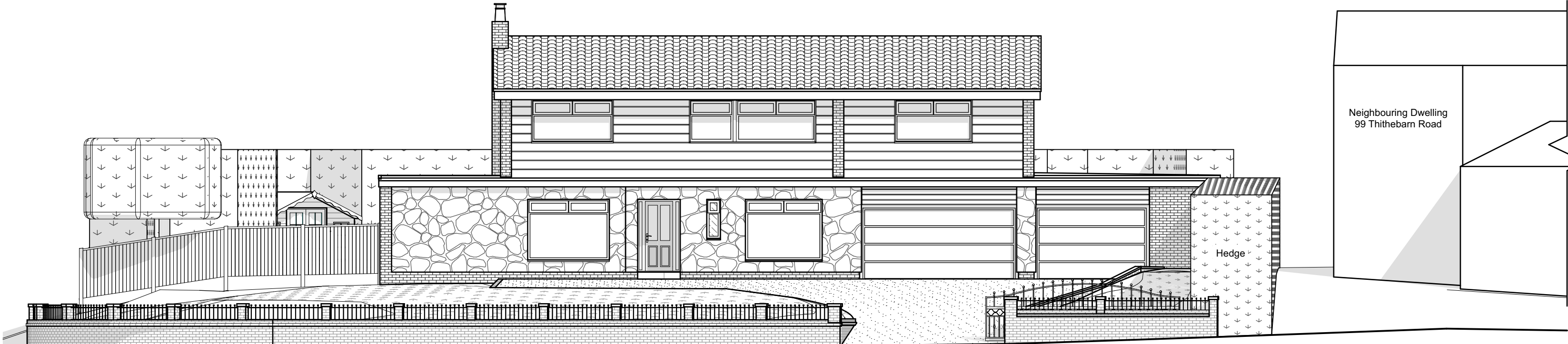
Existing Front Elevation 1:100
