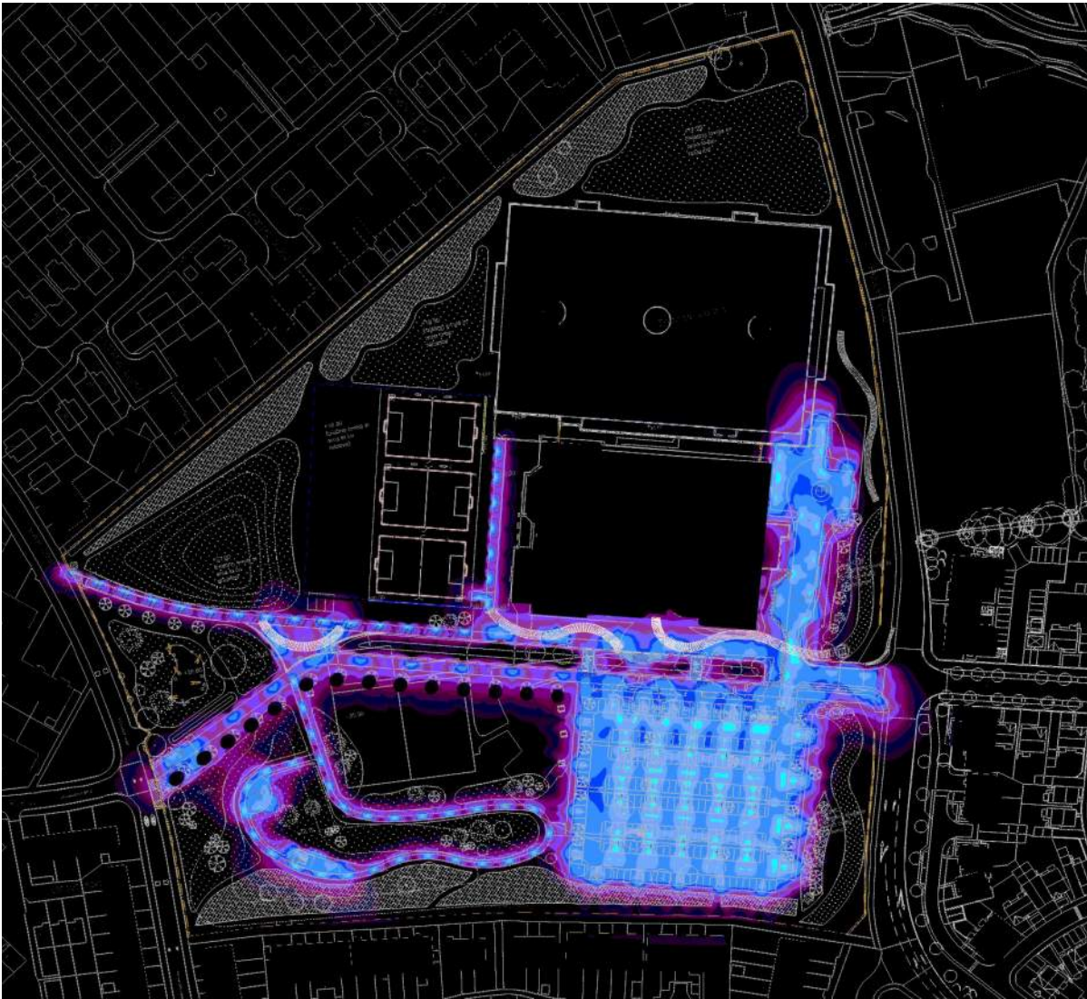
Post-curfew false colour view showing illuminance levels (produced by the lighting calculation model)
